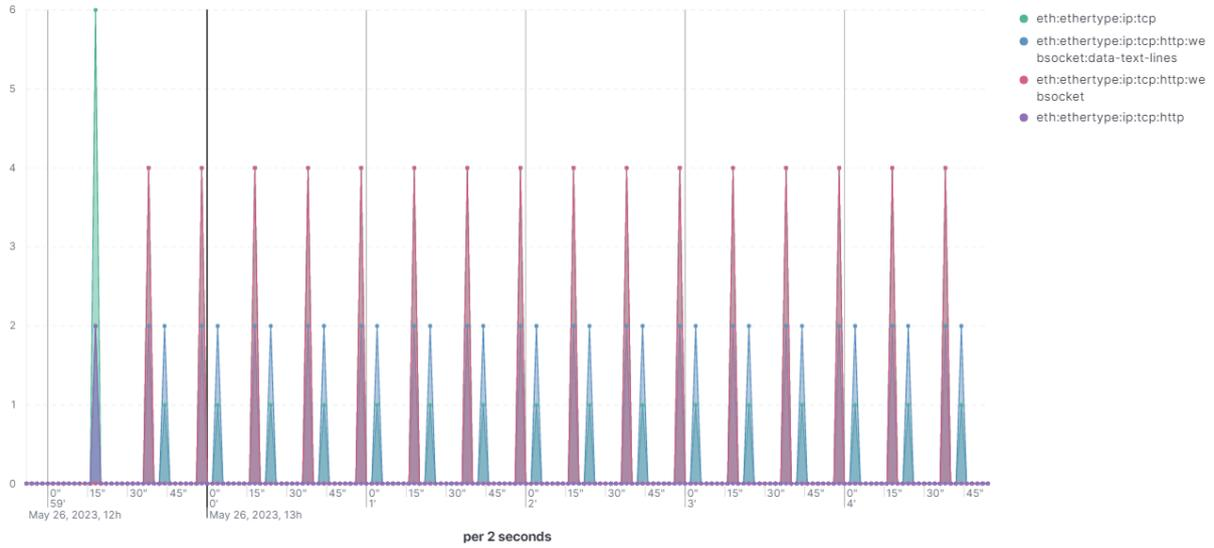
**Figure 10. Count rate of packets (count per 2 seconds), colors correspond to different type of packets sent in the communication between particular a CS and the Controller.**
