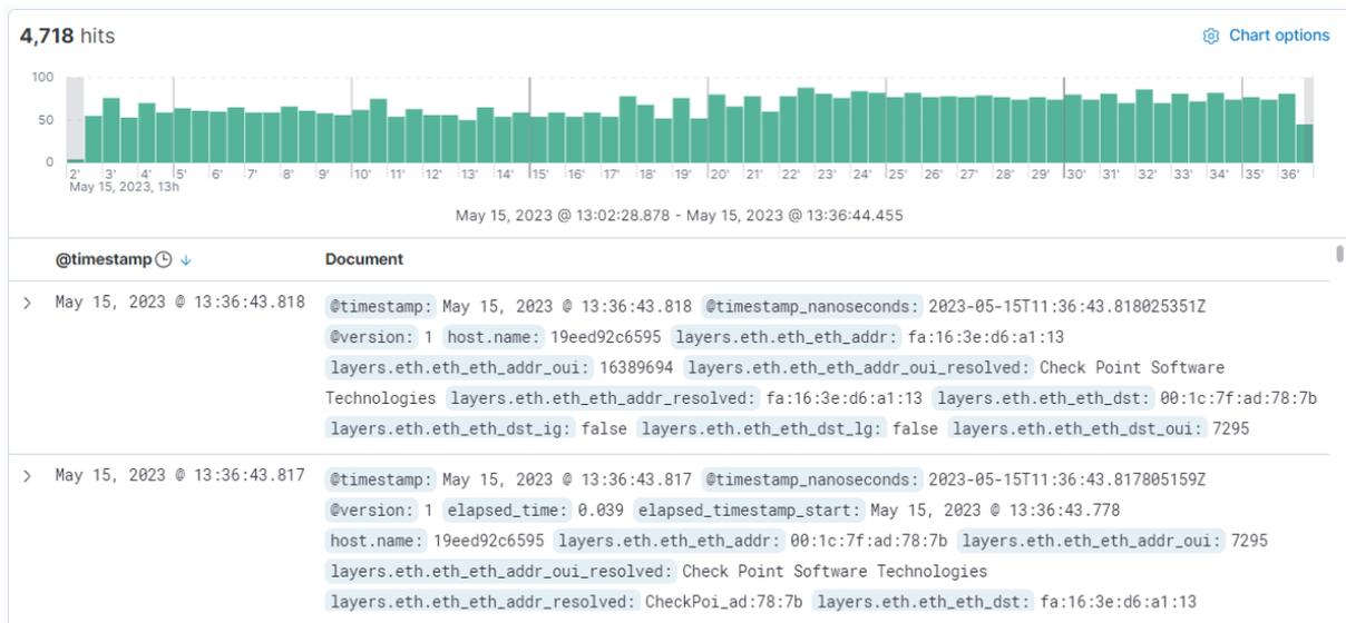
**Figure 8. Snapshot of Logstash pipeline, the bar plot corresponds to the count rate of captured packets from the network, below part of the content of selected packets is shown.**
