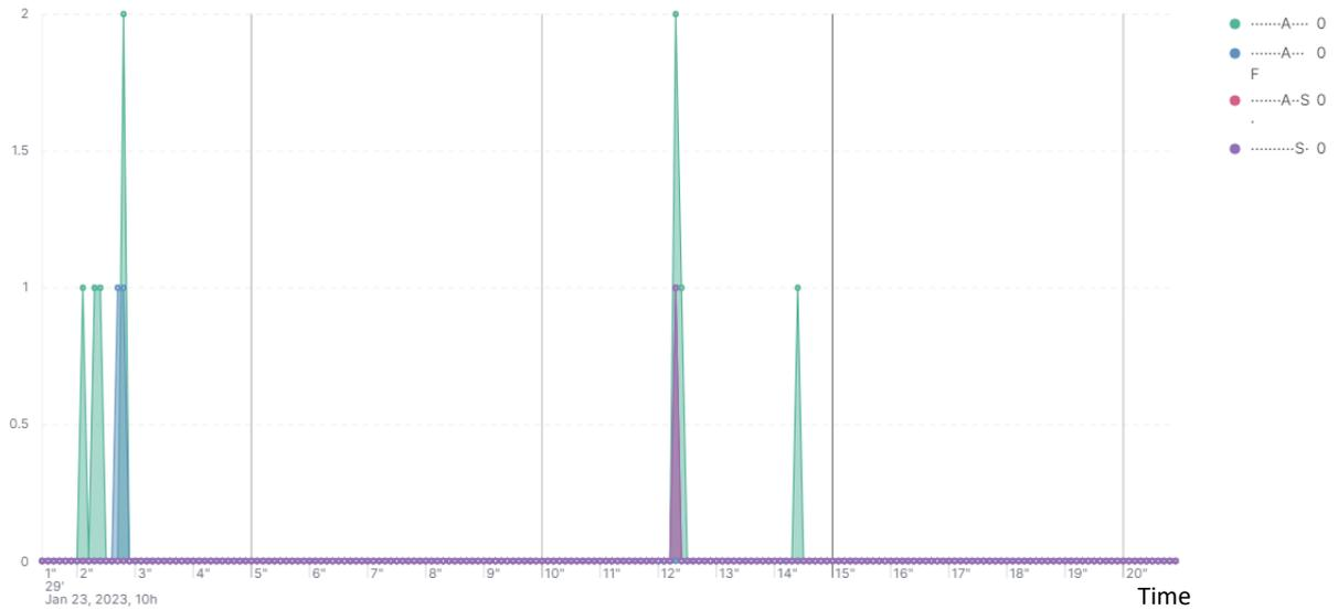
**Figure 11.** Count rate of TCP packets (counts/s) exchanged between a selected CS and Controller during the end of a connection and the start of a new one; colors correspond to different TCP flags.
