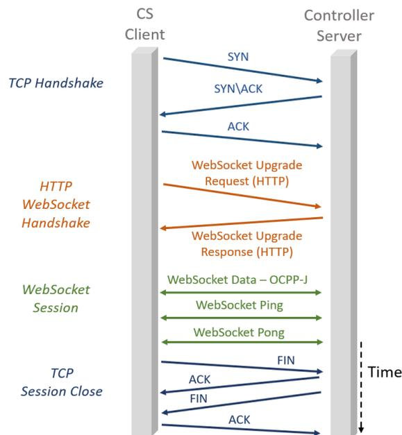
Figure 9. A diagram describing the connection between a CS and a Controller using OCPP-J/WebSocket
